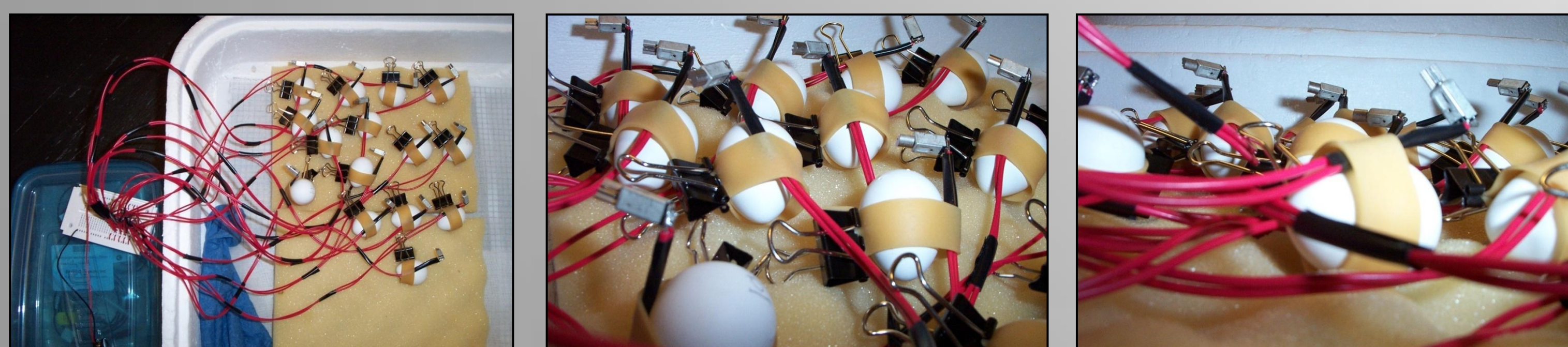
Vibro-tactile stimulation delivered to the embryos via a wire attached to their egg with rubber bands.
